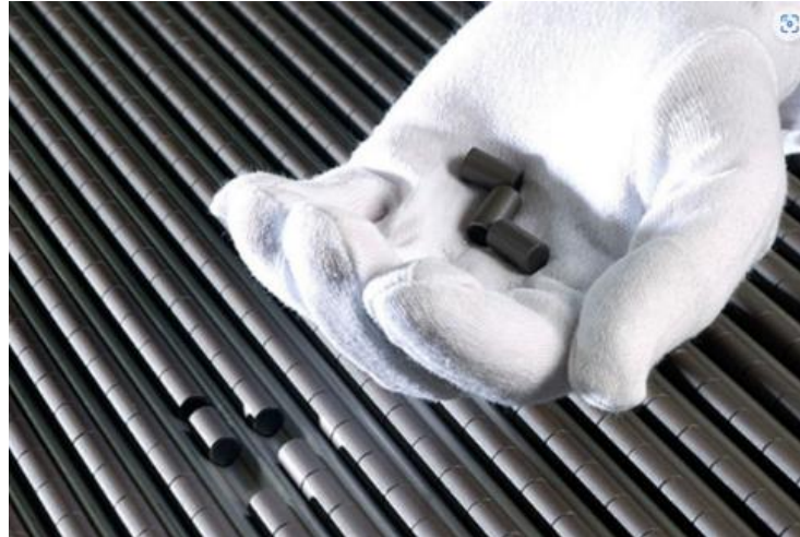
Uranium pellets used in fuel rods
